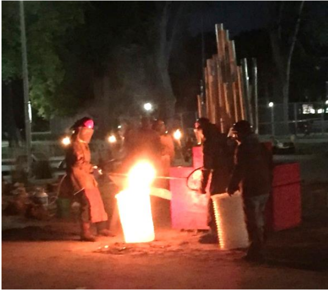
Pouring molten iron into casts.
