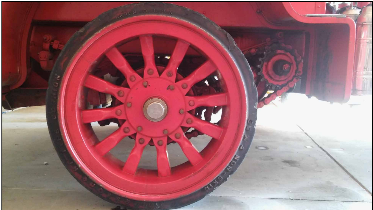
Even though pneumatic tires were available in 1923, the American LaFrance came with hard-rubber tires. The truck is chain-driven.
